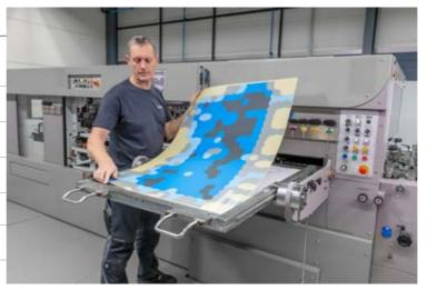
The die-cutting machine is subject to tolerances caused by wear and tear. For this reason, it was previously necessary to fill worn out zones with make-ready paper when setting up an order. This effort was required for every single order. With digital zone levelling, the process is much more efficient. This zone make-ready only needs to be done once. And then holds on for months to come.
