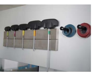
The Marbach Tool Organizer Set 1 keeps your die-cutting machine tidy. It consists of special magnetic rails, which are equipped with wrenches and magnetic hooks for make-ready tapes. For immediate access directly at the die-cutting machine. This reduces walking distances and search times.
