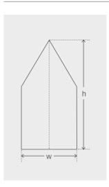
**D – center bevel**The standard for cutting paperboard. Also available as side bevel.
