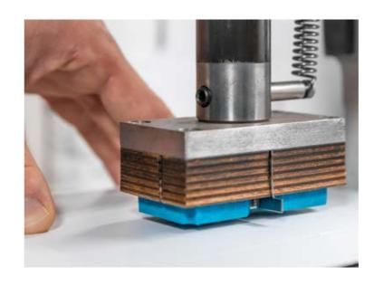
For an easy production of test samples for the crease bend tester it is recommended to use the sample cutter. With this, samples with the size 60 mmx25 mm can be cut. The sample cutter and suitable tools are equipped with a visual aid. This ensures the correct position for cutting the paperboard strips quickly and precisely.
