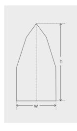
**D4 – long center bevel**For thick materials. The standard for corrugated board. Also available as side bevel.
