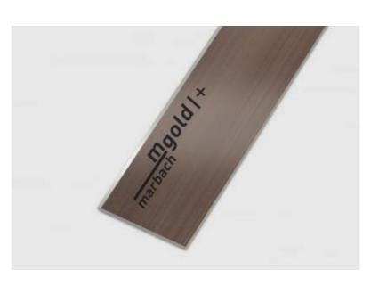
Like its little brother mgold, this cutting rule has a 42° edge. Due to this and its special coating, it is not only very sharp but also very hard and therefore suitable for the highest demands. It is extremely resistant to abrasion and is thus used when maximum tool life is required for die-cutting critical materials.
