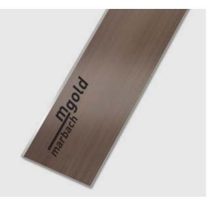
The special cutting rule mgold. Impressive hardness. mgold has a 42° cutting edge. Therefore it is very sharp and works perfectly for cut scores. mgold is optimal for long runs and critical material. Also for cutting metallized cartons and thin metal foils.
